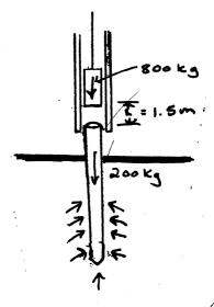
Hammer and Pile move against ground resistance
